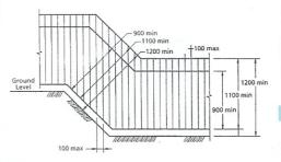
Spacing between vertical uprights must not exceed 100mm at any point.
