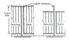
If the latch is on the inside of the fence it should only be accessible by reaching over the top of the fence. On gates of open construction a latch shield will be required.
